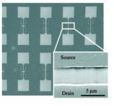
terning of transparent source and drain electrodes. The low-temperature fabrication allowed the researchers to use a similar technique with polyethylene terephthalate (PET) as a flexible substrate. Performance tests showed that the TTFTs on glass substrates had good transparency and high effective mobilities of about 1300 cm<sup>2</sup> V<sup>-1</sup> s<sup>-1</sup>, the highest among transparent transistors using various active materials reported thus far. The TTFTs
