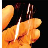
on PET substrates operated successfully when bent up to 120°. As proof of principle, the researchers further utilized the transistors to construct a fully transparent and flexible logic inverter on a plastic substrate, as well as to control commercial GaN light-emitting diodes with light intensity modulation of 10<sup>3</sup>. The results suggest that aligned nanotubes could form the building blocks for future high-performance transparent and flexible electronics.
